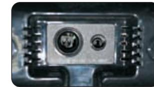
2. **Keyboard Connection:** Connect the Vu wireless keyboard USB dongle to the MCU Codec as shown.
