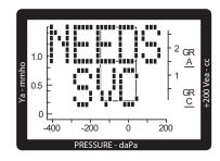
The NEEDS SVC message appears when something has caused the tympanometer to fail an internal test. The NEEDS SVC message will display for approximately three seconds; then the device will power down. Return the tympanometer to a Welch Allyn service location for service. (See Service information.)
