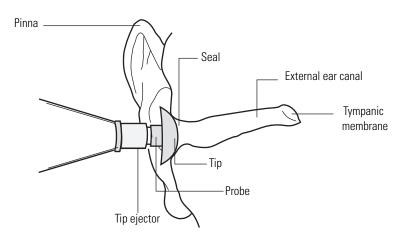
2. Push the tip onto the probe, making sure that the tip is fully seated.
