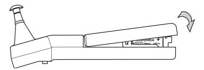
5. Tighten screw in clockwise direction. To avoid stripping the screw threads, do not tighten excessively.
