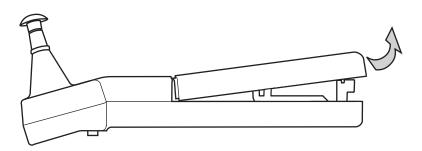
4. Push down on the positive (+) end of the battery. The battery will eject.
