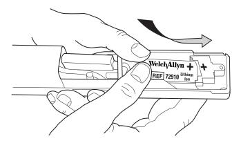
4. Replace the cover by inserting the tip end under the front cover, lowering the opposite end, and replacing the screw.
