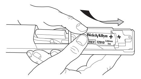
6. Replace the cover by inserting the tip end under the front cover, lowering the opposite end, and replacing the screw.
