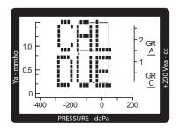
Welch Allyn recommends annual calibration of your tympanometer to ensure equipment accuracy. The CAL DUE message will display each time the device is powered on when one year has passed since the last calibration. Press and hold the TEST button for approximately two seconds to clear this message and resume patient testing or print information stored in the Handle.
