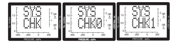
The SYS CHK (SYS CHK0, SYS CHK1) message indicates that the Handle is doing a self-check to ensure proper operation. The Handle will shut off upon completion of the test. Press any button to power the Handle and clear the condition.
