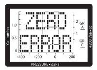
The ZERO ERROR message indicates that a large pressure change occurred during automatic pressure compensation at the start of a test. If this message appears, press the TEST button and start the test again.
