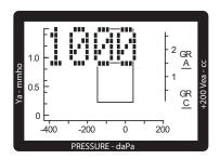
These messages indicate the unit's frequency options. You can toggle between frequencies by simultaneously pressing both the  $\overline{\mathbb{R}}$  Right memory and  $\overline{\mathbb{Q}}$  Left memory buttons.
