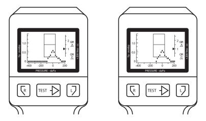
For 1000 Hz, the test is complete when one of two "Quick-Interpretation" messages appears—either PASS or REFER—as shown in the examples below. If patient or instrument movement causes a leak beyond -300 daPa in 1000-Hz mode, the test will be stopped but the data will be saved.
