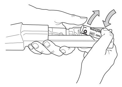
5. Insert the new battery by placing the positive (+) end of the battery against the contact in the holder. Push the battery lightly to compress the contact, and lower the battery into the compartment.
