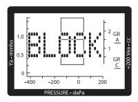
The test cannot continue since the measured admittance is less than 0.2 mmho.
